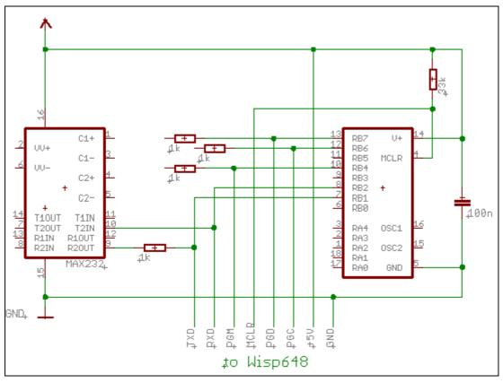
Figure 1 : combination of RS232 interface and serial pass-through
