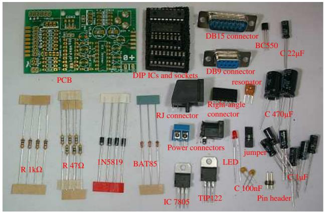
Place and solder the three BAT85 diodes. The (black) band on the diodes must be at the side of the white band in the PCB silkscreen (white print on the PCB). Trim the wires.
