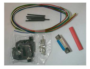
Strip a few millimeters of the six colored wires and solder them to the female DB015 connector. The solder cups are numbered from left to right: 1 ... 8. You use only the top row, the bottom row has only 7 cups. From left (1) to right (6) the wire colors are black, red, green, blue, yellow and white.
