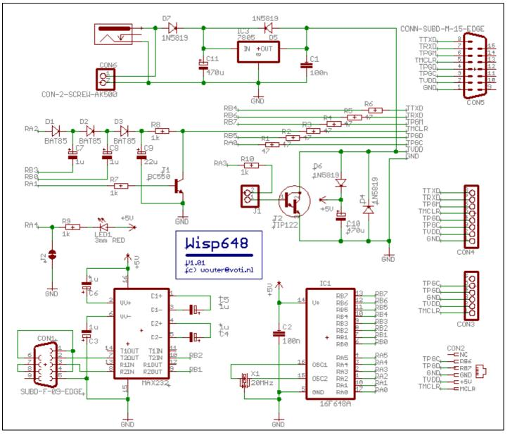
Figure 2 : Wisp648 circuit diagram
